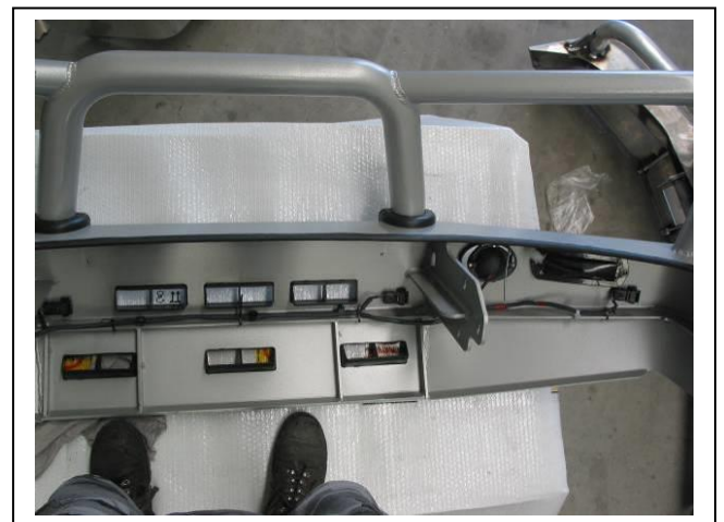
Figure 10: Parking sensor mounted into protection bar with secured wiring.
