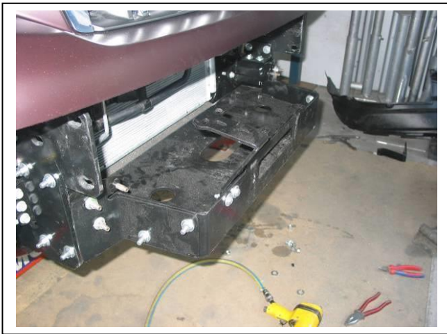
Figure 7: Winch frame fitted to chassis rails
